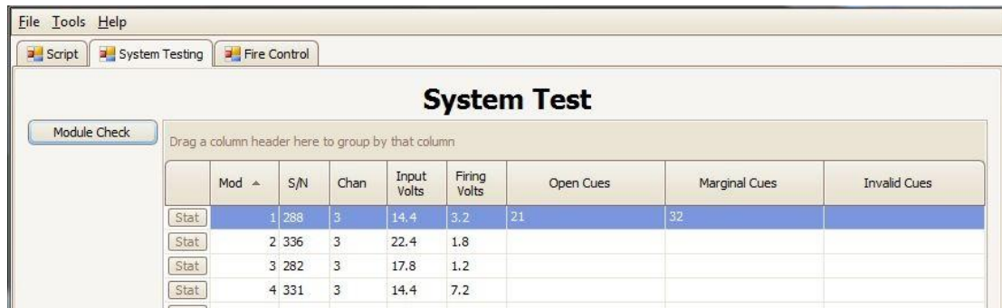
Figure 28: Scripted Show - Continuity Check Through the Software
